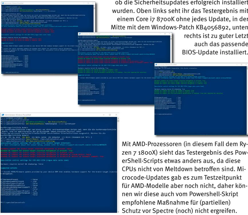
The screenshots show the output of the PowerShell script. The top window shows a Core i7 8700K without updates, with some Spectre Variant 2 and Meltdown entries in red (no protection). The middle window shows the same system after Windows patch KB4056892, with all entries in green (protection active). The bottom window shows the system after the BIOS update is installed, also with all entries in green.
